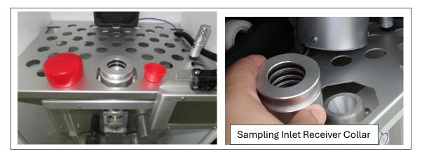
12. Slide the inlet downtube through the inlet pipe flange (through the black sealing ring or pipe seal) on top of the enclosure until you can see it inside the enclosure.
