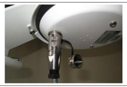
21. Route the sensor cable to the back of the enclosure and attach it to the connection labeled as EXTERNAL AMBIENT SENSOR.
